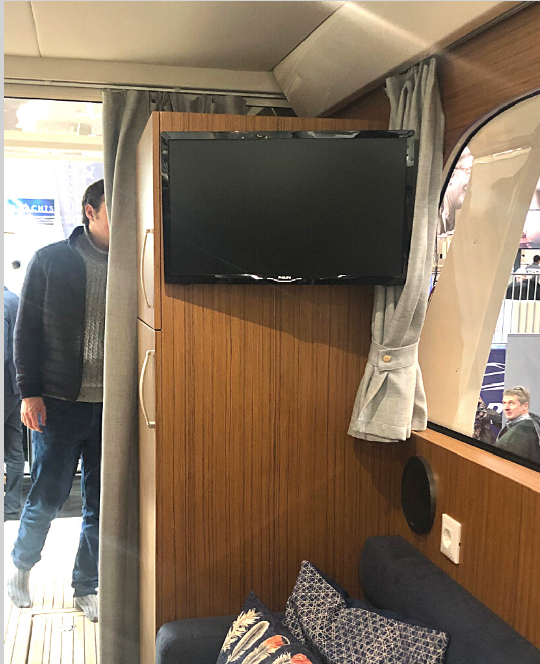
LED LCD TV 24" DVBT in the salon - mounted and prewired TV antenna for digital / analog signals
