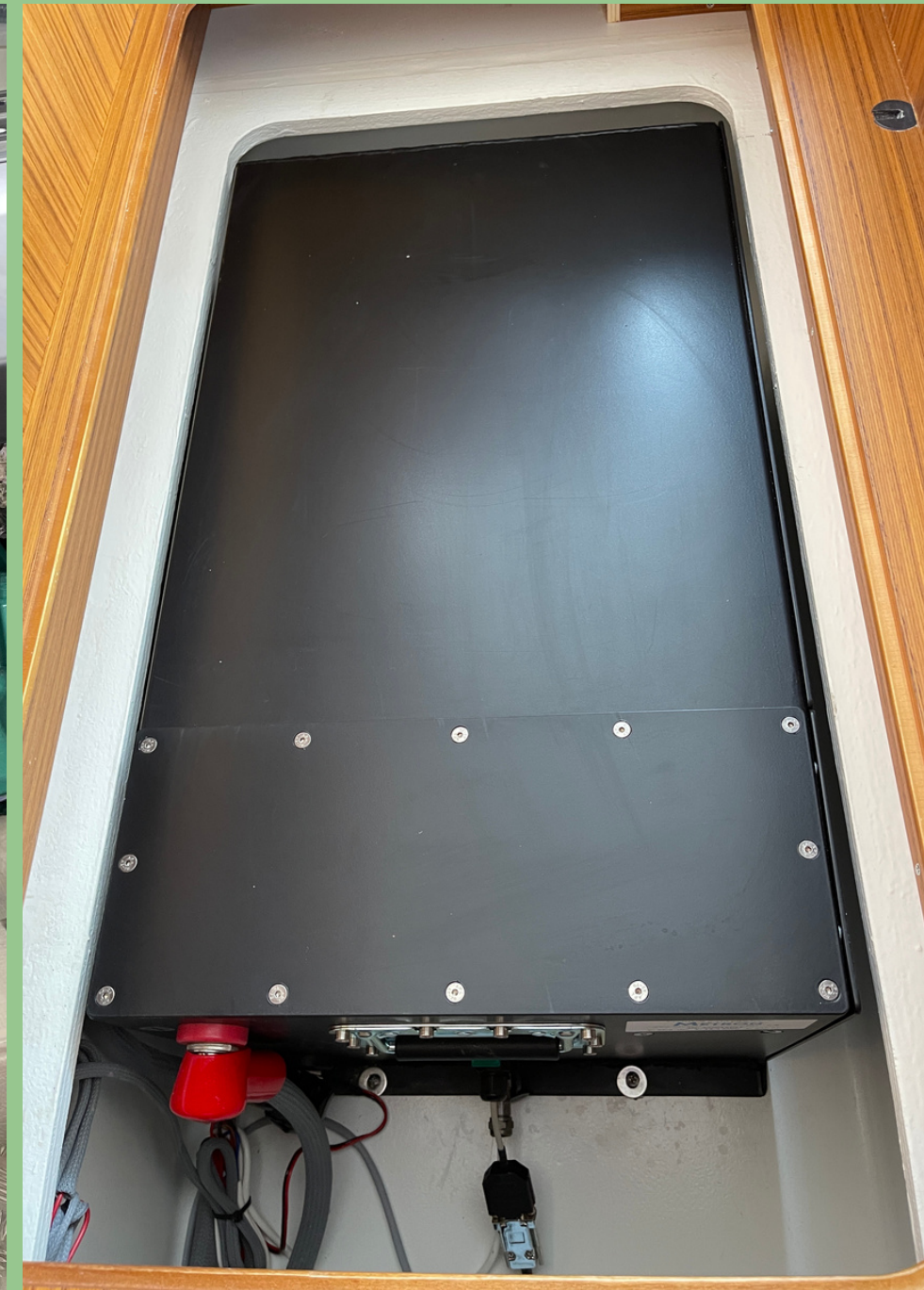
Lithium-Polymer battery 1 x 13.3 kW/h (maximum 1 additional unit)
