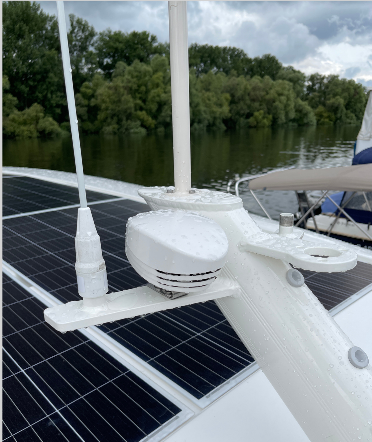
HORN ON RADAR MAST
